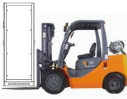
Figure 4-1 Moving method for cabinet
