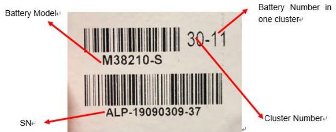
Figure 4-9 Diagram of the Battery SN
